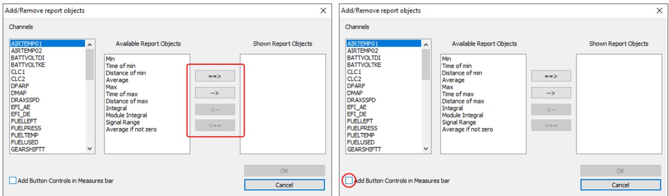
Checking "Add Button Controls in Measures bar" (right image below), an icons bar appears next to each channel name in the main page left tab allowing you to show/hide max/min value just clicking on the proper icon (
