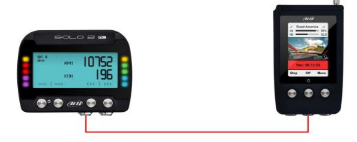
To connect Solo 2 DL to LCU-One CAN connect 5 pins Binder connector placed bottom left of Solo 2 DL to 5 pins Binder connector of LCU-One as shown here below.
