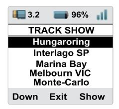
To switch to MANUAL mode press "Change" in Auto mode and "MANUAL SEL" enables. If a track has been selected it will be shown with the related distance form current position (Silverstone GP, 679 miles away in the left image below). To select another track press "Sel" and the list of all track loaded in your SmartyCam HD will be shown.
