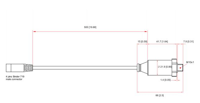
The sensor ends with a 4 pins Binder 719 male connector. The image below shows the connector pinout from solder termination side.
