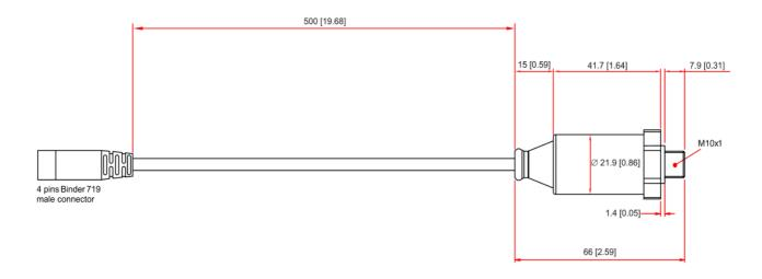
The sensor ends with a 4 pins Binder 719 male connector. The image below shows the connector pinout from solder termination side.
