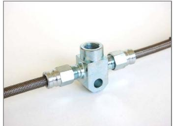
Install the sensor on the junction wrapping the thread with Teflon to guarantee its tightness.
