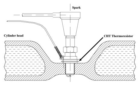
Figure 2: Cylinder head Thermoresistor installation
