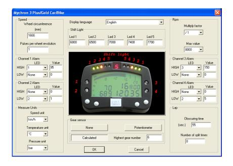
Wheel circumference: this function allows the user to set wheel circumference (in mm or in inches); this value is fundamental to correlate the wheel revolution speed and the vehicle speed.
