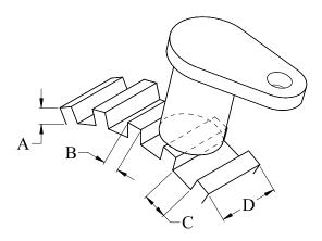
In the following table it is reported a short description of the minimum values for the trigger dimensions A, B, C and D required for a correct sensor's working.
