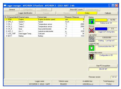
Attention: if the gear channel and the accelerometer one have not been correctly calibrated, it will not be possible both to acquire the current gear and, for MyChron 3 Gold/Gold XG only, to create the circuit map. It is recommended to pay a particular attention when calibrating/autocalibrating the channels.
