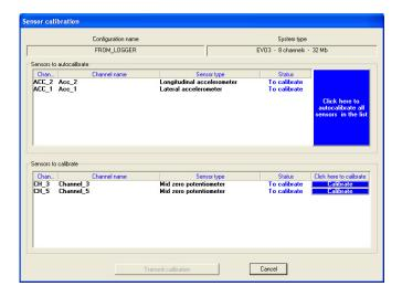
The g-force sensor, the gyroscope and the "potentiometer distance" need to be autocalibrated pressing button "Click here to autocalibrate all sensors in the list". Once autocalibrated, the "calibration status" will turn from "To calibrate" in "Calibrated".
