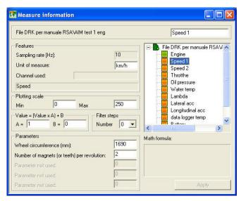
If you choose a channel from the channel list in the right upper corner list, it will also appear the parameters (in the lower left corner) that the user can set (i.e. RPM multiply factor, wheel circumference, pulses per revolution, etc...)
