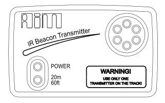
The transmitter has two operating modes: *Low* power and *High* power. The Low Power Mode has to be used when the track is less than 10 meters wide, while the High Power mode has to be used when the track is wider than 10 meters.
