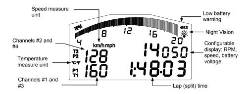
The wide display with backlight shows RPM (graphical bar), temperature and pressure analog inputs, test and lap number and, when the vehicle passes in front of the beacon, it shows the Lap Time (or Split Time). It is also possible to configure a second display page (using button **VIEW**) in order to see the RPM digital value (as shown in the previous drawing), the vehicle speed (in km/h or Mph) or the best lap time. When you are not running it is also possible to see the battery voltage.
