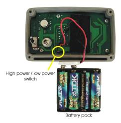
Please, remember that, in High Power Mode, the transmitter has to be powered by an external 12 Volts battery.
