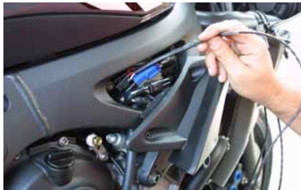
Figure 22: installing the water temperature and the speed connectors.
