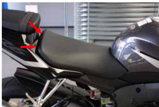
Figure 1: location of the seat screws.
