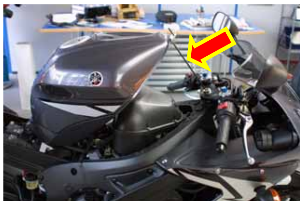
Figure 3:Uplifting the gas tank.
