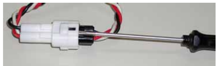
Figure 16: How to unplug a connector
