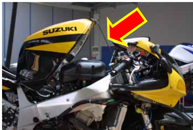
Figure 8: Uplifting the gas tank
