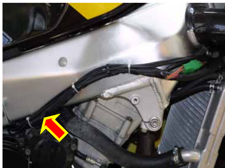
Figure 21: Wiring installation – run the wiring along the chassis
