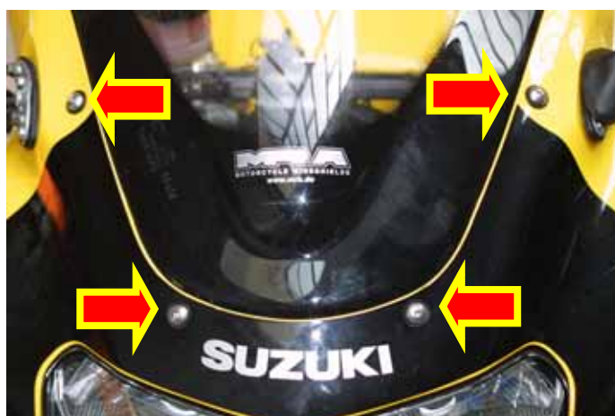
Figure 1: Front fairing – 4 mm hex screws
