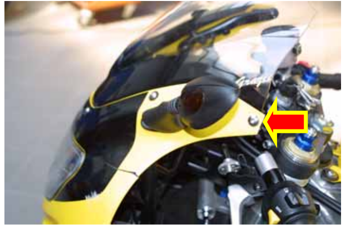
Figure 2: Front fairing – 5 mm hex screw
