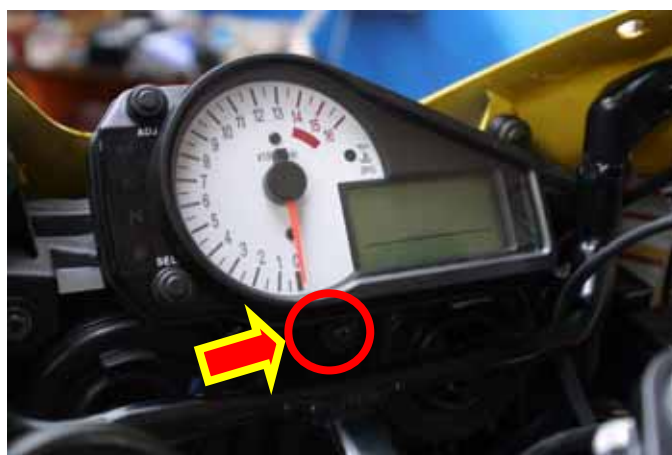
Figure 9: Removing the screw from the stock dash
