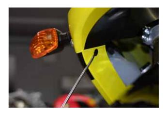
Figure 7: removing the plastic pin
