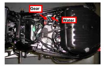
Figure 17: on board connectors - Water temp. / Gear
