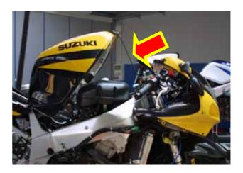
Figure 11: Uplifting the gas tank
