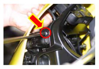
Figure 30: fixing the lateral screws
