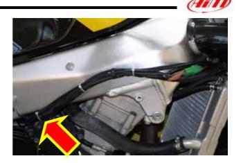
Figure 25: Wiring installation – run the wiring along the chassis
