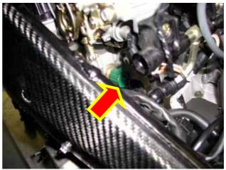
Figure 19: Water temperature connector – particular
