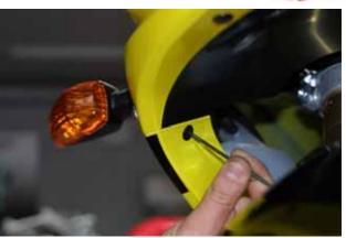
Figure 6: Unlocking the central clip of the plastic pin.
