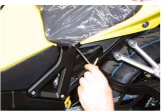
Figure 9: Unscrewing seats screw
