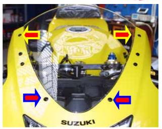
Figure 3: Front fairing – 4 Phillips recess screws.
