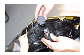
Figure 26: Wiring installation – particular of the AMP connector
