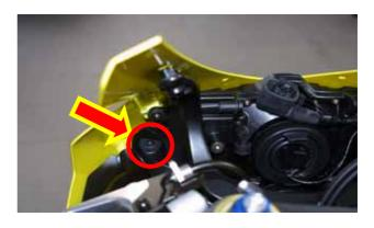
Figure 12: position of fairing and headlight screws
