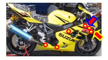
Figure 4: Right lateral fairing – screws/pins location
