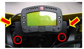
Figure 28: Kit correctly installed
