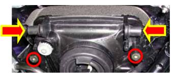
Figure 29: position of the 4 screws.
