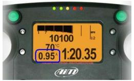
Switching **EVO3 QM** on Lambda controller is recognised at start up and probe warm-up procedure starts. During this period the controller takes the probe to its working temperature (until around  $780 \,^{\circ}\text{C} - 1436 \,^{\circ}\text{F}$ ).
