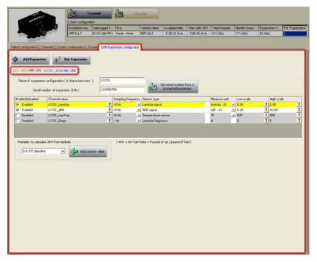
In case serial number has not been get, press "Get serial number from a connected expansion" button.
