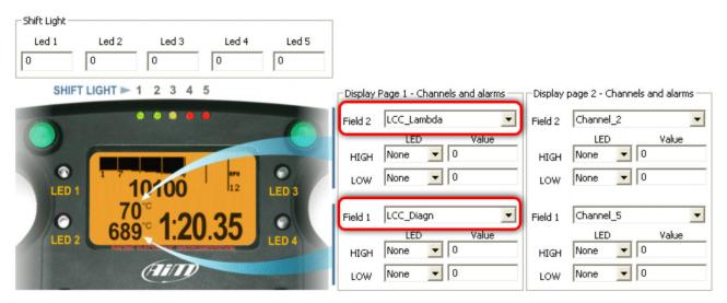
**Note**: LCC\_diagnosys channel shows **LCU-ONE** working status and can show up to four messages:
