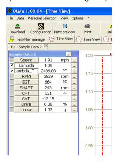
To better analyse carburetor values we would suggest to show XY diagram of Lambda probe with RPM values on abscissa axle and Lambda values on ordinate axle. This way a more immediate reading of carburetion status is available.
