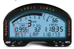
Powering MXL QM and Lambda controller on at the same time, LCU-ONE CAN is recognised at start-up and probe warm-up procedure starts. During this period the controller takes the probe to its working temperature (until around 780  $^{\circ}$ C – 1436  $^{\circ}$ F).
