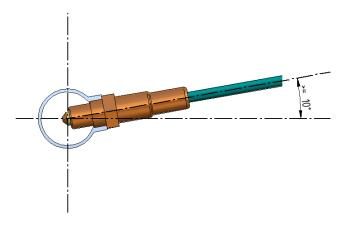
When the probe has been installed, do not let the cable pass close to heat sources (the exhaust pipe for example).
