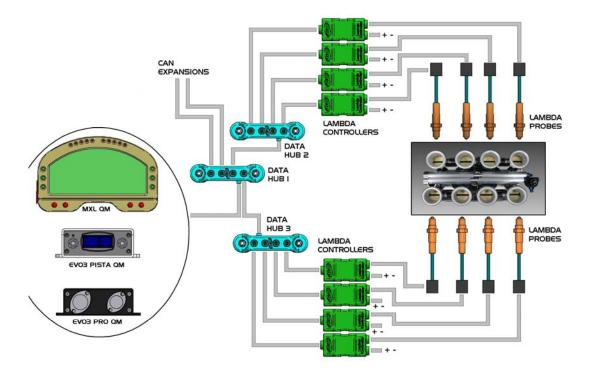
Each Lambda controller has to be connected to the battery.
