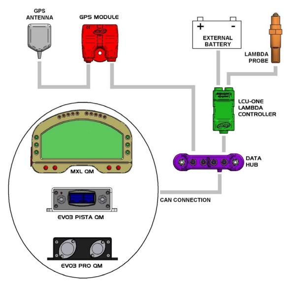
Lambda controller connection to other CAN peripherals scheme is shown above. We suggest to insert a 10 A fuse in series between External Battery and Lambda controller to protect the latter.
