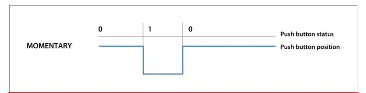
Please note: only setting the pushbutton as Momentary, you can associate a command to each pushbutton but to do so it is necessary to have previously added a Display to PDM configuration.
