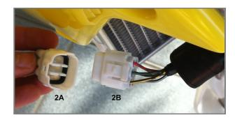
Plug AiM cable (1) in the connectors shown here above (2a and 2b) as in the scheme below. This way you can continue managing different Suzuki original ECU maps.
