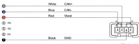
4 pins FCI 4 male connetor pinout contact insertion view
