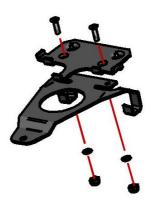
Remove the steering wheel dumper starting with the Uniball screw highlighted here on the right.
