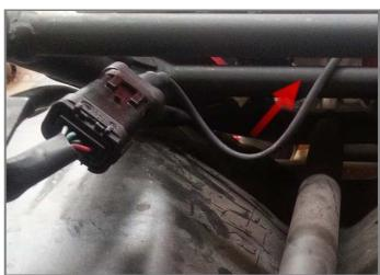
To reach SoloDL make the cable pass between the fuel tank and the bike frame.
