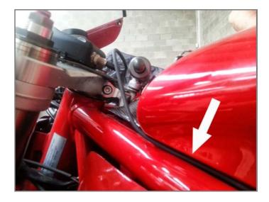
Connect the cable to SoloDL as here on the right.
