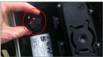
Connect AiM wiring to BMW wiring as highlighted on the right.
