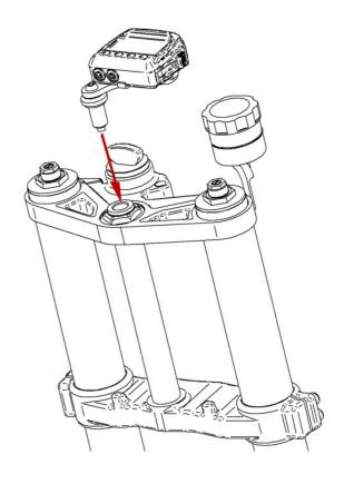
Tighten the central screw on the hinge so that this last grips.
