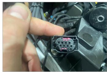
models from 2024 have this connector placed on the tail of the bike under a cover, as shown here on the right.
