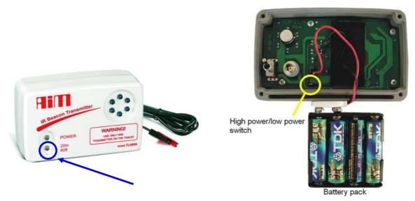
The transmitter can be internally powered using 8 batteries to be inserted in the proper case (unscrew the transmitter case backside and insert them in), or externally powered using a 12 Volt power source to be connected to the battery through the power cable. It is suggested to prefer external power.
