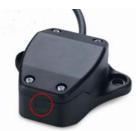
Warning: the receiver needs to be installed so that its "eye" (circled in the image above), sees the transmitter.
